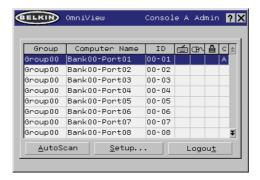
The Setup page is only available to the Admin user and is used to set the group name, computer name, and computer scan times. The scan time is dependent on the port being scanned, and is global (i.e. it's independent of the console or user). While scan times are independent of the user, AutoScan will skip computers that the user does not have permission to view.
